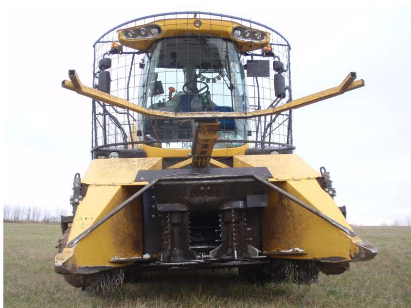
Forage harvester with special cutting head for coppiced trees (max. diam. 10-15cm)
