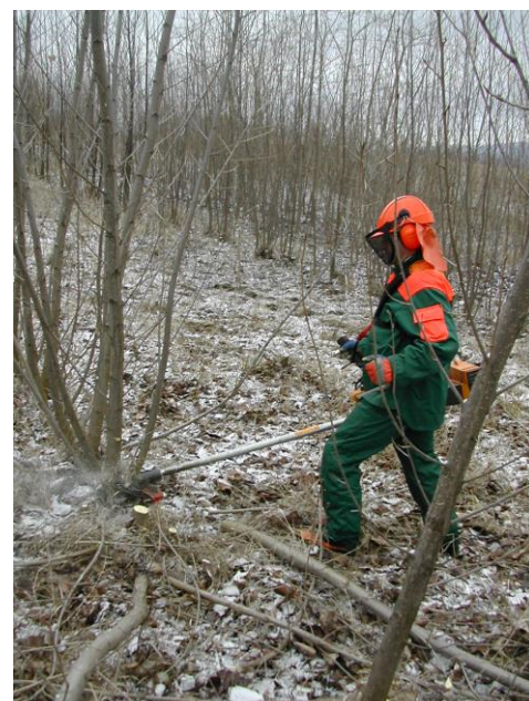
Brush cutter used for manual 2-phase harvest of coppice tree line/belt (max. diam. 10-15cm)
