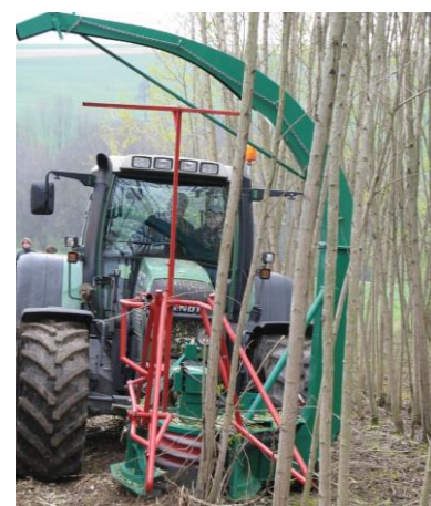
Mower-chipper harvester on tractor for harvest single line of coppiced trees (max. diam. 15-20cm)
