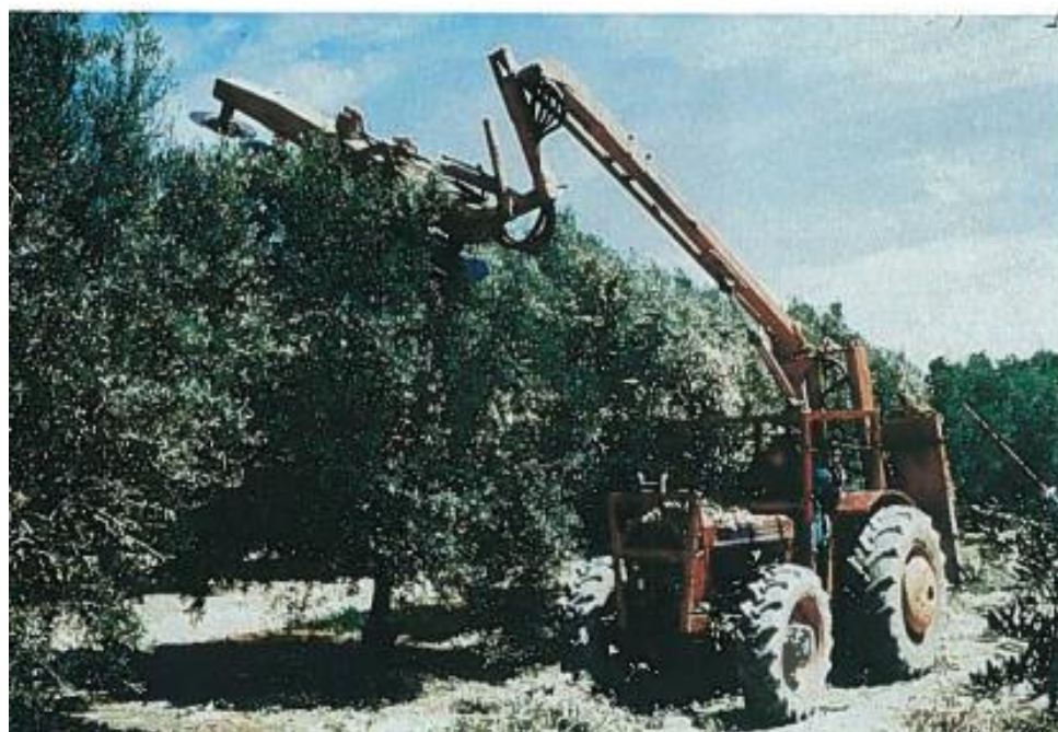
Different methods of orchard pruning, from left to right: manual pruning using motorized machinery and mechanical pruning using steel toothed discs on the arm coupled to the tractor. Source: Agronomy and pruning of olive groves, Junta de Andalucía.
